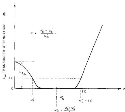
Fig. 2. Definition of response parameters for low-pass impedance-transforming filters. (The frequency scale for the tabulated design is normalized so that  $\omega_b' = 1$ , as indicated above.)
