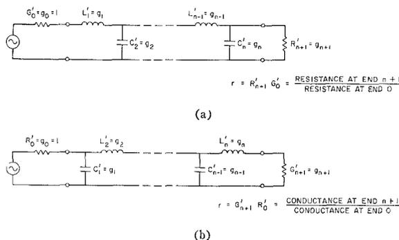
Fig. 1. Definition of normalized prototype element values for impedance-transforming networks of low pass filter form. (The tabulated element values are normalized so that  $g_0 = 1$  and  $\omega_b' = 1$ , as in Fig. 2.)
